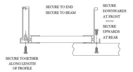
Lift a further pre-assembled panel on to the roof and locate onto the previously fixed Aluminium profile. Secure as above using fixings supplied.
