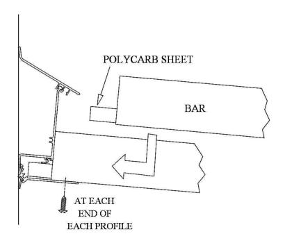
Secure the panel along its length to the Left Hand End Closure. At each end secure to wall plate and support frame, fixing upwards into the wall plate and downwards into the eaves beam.
