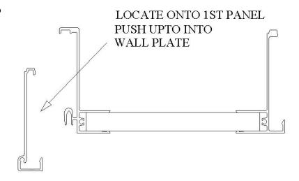
Each glazing panel has a polycarbonate protrusion of approximately 25mm this needs to be fed into the wall plate to provide a watertight seal.
