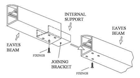
Please ensure the Eaves Beam is installed with the slope away from the wall.(See diagram)
