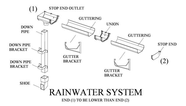
As a general guide the minimum fall for the gutter is 1:600 which equates to a fall of 10mm in a 6m length.
